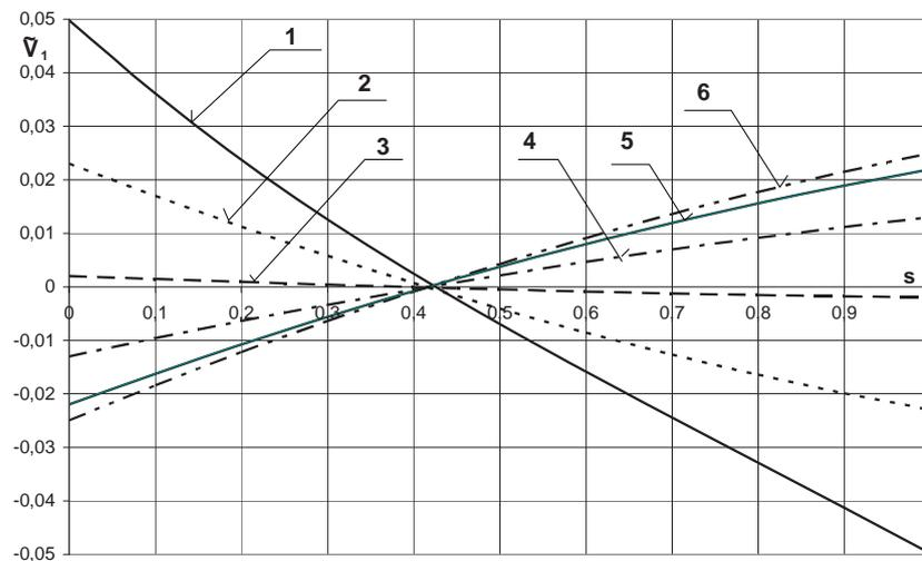
Fig. 3. Velocity distribution  $\tilde{V}_1$  in the circumferential direction by velocity perturbations  $V_{10} = 0.05, V_{1h} = -0.05$ , in gap height  $s$ , in the time  $t_1$ : 1) 0; 1, 2) 0.1; 0.9, 3) 0.2; 0.8, 4) 0.3; 0.7, 5) 0.4; 0.6, 6) 0.5
