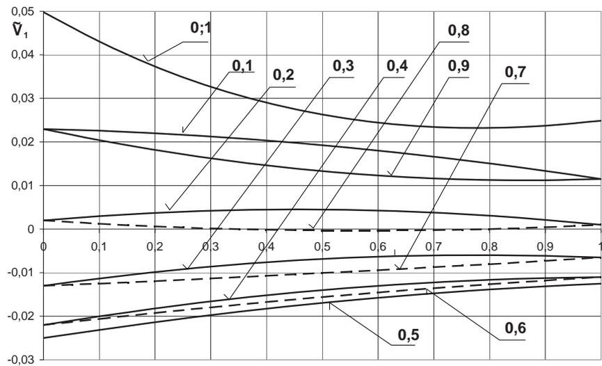
Fig. 2. Velocity distribution  $\tilde{V}_1$  in the circumferential direction, in gap height  $s$ , in the time  $t_1$  by velocity perturbations  $V_{10} = 0,05, V_{1h} = 0,025$
