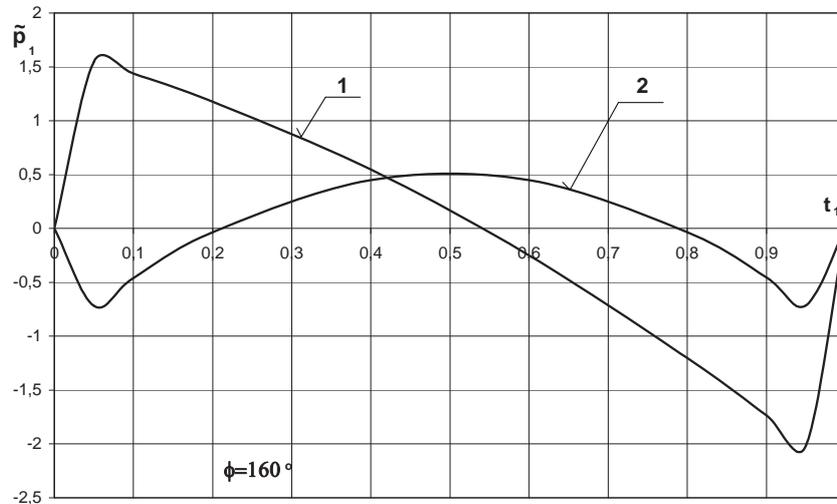
Fig. 1. Pressure distributions  $\tilde{p}_1$  in place  $\varphi=160^\circ$  in the time  $t_1$  by velocity perturbations: 1)  $V_{10}=0,05$ ;  $V_{1h}=0,025$ ; 2)  $V_{10}=0,05$ ;  $V_{1h}=-0,05$
