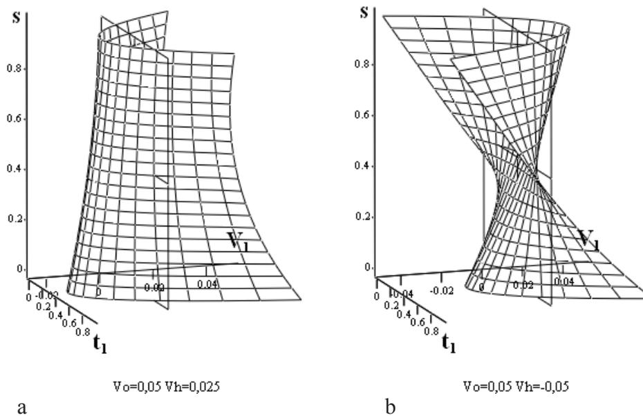
Fig. 4. Velocity distribution  $\tilde{V}_1$  in the circumferential direction in gap height  $s$  in the time  $t_1$ , by velocity perturbations a)  $V_{10} = 0,05$ ,  $V_{1h} = 0,025$  ; b)  $V_{10} = 0,05$ ,  $V_{1h} = -0,05$
